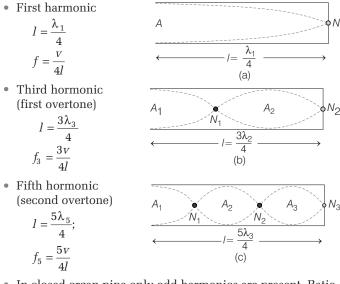
In closed organ pipe only odd harmonics are present. Ratio of harmonic is n<sub>1</sub>: n<sub>3</sub>: n<sub>5</sub> = 1:3:5.
